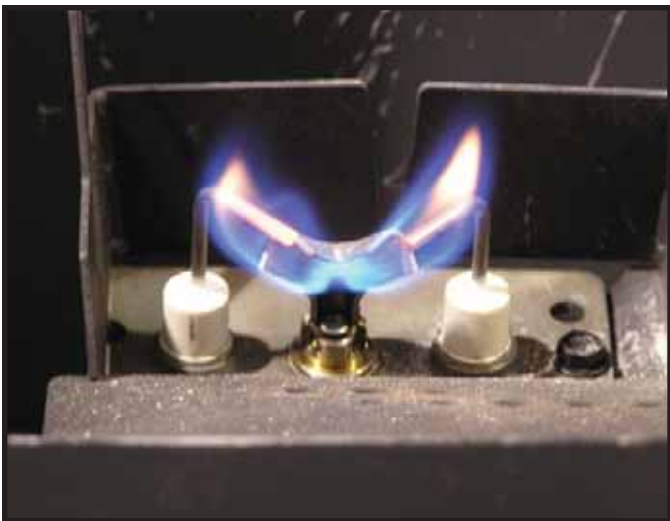
Figure 3.2 IPI Pilot Flame Patterns
